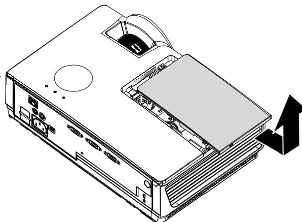
**3.** Remove the three screws from the lamp module.
