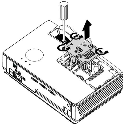
**6.** Reverse steps 1 to 5 to install the new lamp module. While installing, align the lamp module with the connector and ensure it is level to avoid damage.
