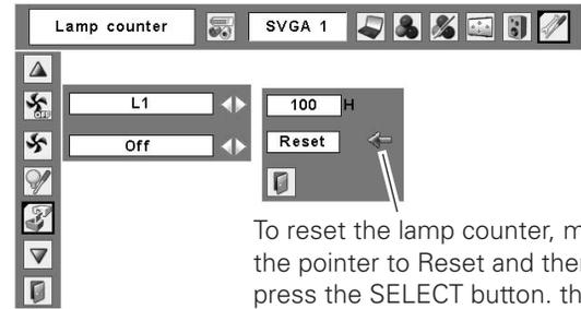
To reset the lamp counter, move the pointer to Reset and then press the SELECT button. the "Lamp replacement counter Reset?" dialog box appears.
